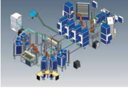
KGHM Polska Miedź S.A. Automatic laboratory for geological and concentrate copper samples (Polkowice, Poland)
