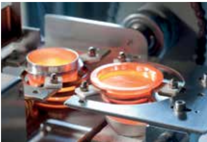
Operating sequence in the fusion module with induction heating in the crucible, ...
