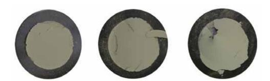
Fig.1: Pressed pellets of different lime samples several hours (~12 h) after the preparation exposed to room humidity. They burst after moisture uptake. Without the addition of HMPA 40 with a wax portion will burst even after some minutes.
